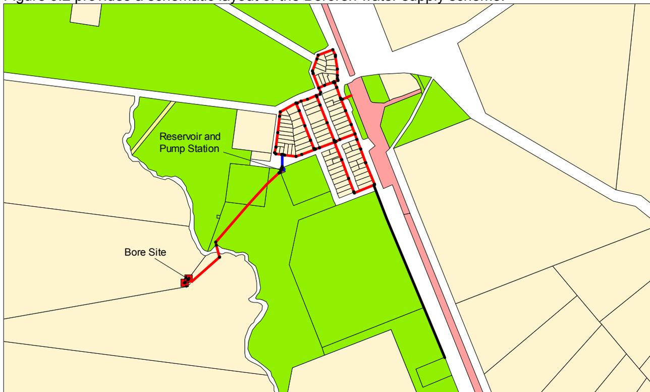
**FIGURE 3.2 : Bororen Water Supply Schematic Layout**
