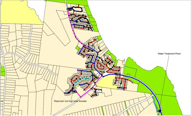
Figure 3.1 provides a schematic layout of the Agnes Water water supply scheme.
